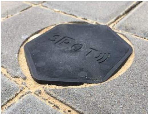
SPOT is a technology platform that uses data transmission via IoT networks to solve parking difficulties. It consists of #Detector (vehicle detector) that reliably tracks parking occupancy in particular slots, #Permit card that validates parking through a cloud-based server application. See below a technical specification of the #Detector.
